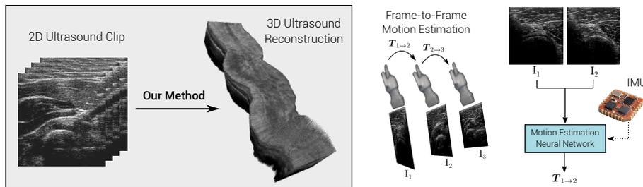
Figure 1: Our system turns 2D standard ultrasound clips into 3D volumes. The method is based on a frame-to-frame motion estimation performed by a neural network with the help of an IMU.
