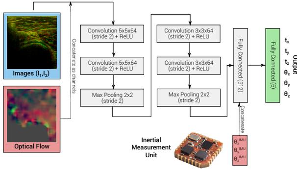
Figure 2: Architecture of our convolutional neural networks.
