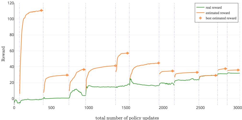
Figure 5: Predicted and real performances during the training process using our approach with one model instead of an ensemble in Swimmer. The policy overfits to the dynamics model which degrades the real performance.
