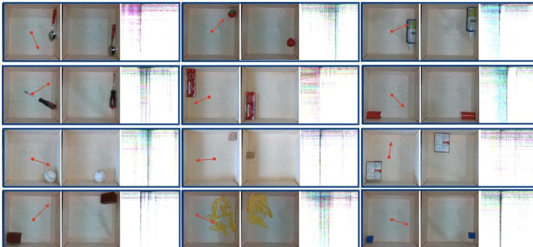
Figure 2: Here are 12 interactions collected using Tilt-Bot. Each interaction is visualized as three images. The left image shows the visual observation of the object before the action is applied along with the applied action. The middle image shows the visual observation after the interaction, while the right image shows the STFT representation of audio generated by 3 of the 4 microphones.
