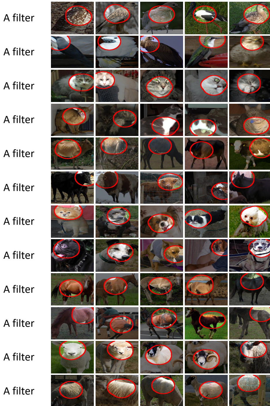
Figure 10: We visualized interpretable filters in the top conv-layer of a CNN, which were learned based on (Zhang et al., 2018b). We projected activation regions on the feature map of the filter onto the image plane for visualization. Each filter represented a specific object part through different images.
