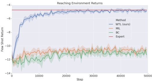
Figure 4: Average return of each method on held out meta-test tasks in the reaching environment, after one demonstration and one trial. Our Watch-Try-Learn (WTL) method is quickly able to learn to imitate the demonstrator. Each line shows the average over 5 separate training runs with identical hyperparameters, evaluated on 50 randomly sampled meta-test tasks. Shaded regions indicate 95% confidence intervals.
