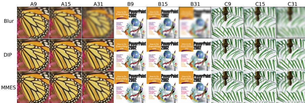
Figure 8: Comparison of our approach with DIP for deconvolution/deblurring task. Three color images were blurred by three Gaussian windows of different sizes. These were recovered by the DIP and the proposed MMES.
