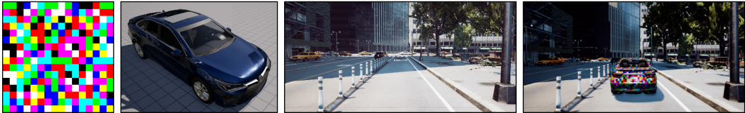
Figure 2: Example procedure of a transformation t . From left to right: a 16 \times 16 camouflage, a high-fidelity vehicle, a location in our simulated environment, and an image due to this transformation over the camouflage.
