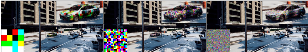
Figure 8: Visualization of three random camouflages of resolutions 4 \times 4 , 16 \times 16 , and 256 \times 256 , respectively, as well as the resulting images by the same camera.
