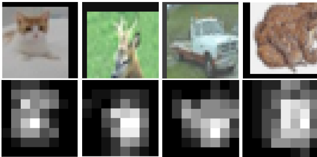
Figure 5: Visualization of gating ratio – Top: feature maps from the final precision gating block in ResNet-20 on CIFAR-10. Bottom: ratio of computing using a high-precision (brighter pixel means higher ratio). PG effectively identifies the location of the object of interest and increases bitwidth when computing in this region.
