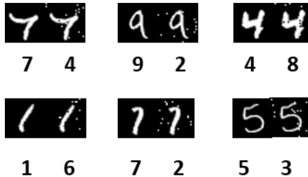
Figure 14: MCTSbug Generated adversarial samples on MNIST dataset. For each pair, left side is the original sample, right side is the corresponding adversarial sample
