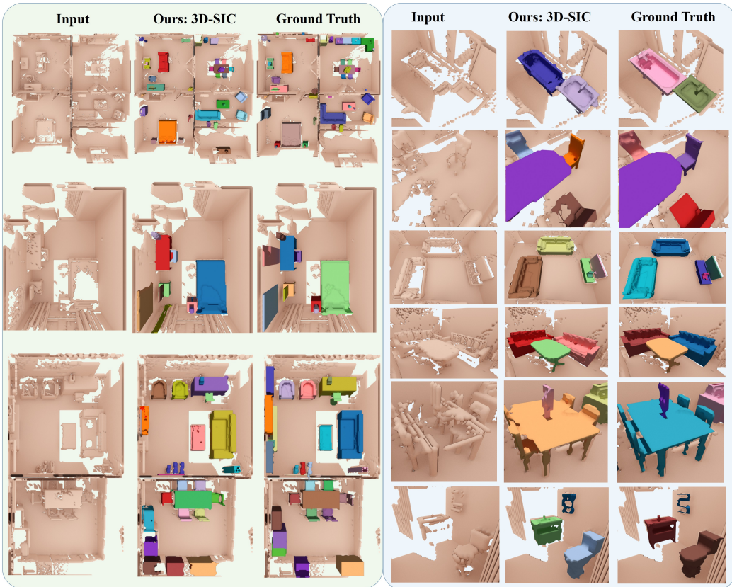
Figure 4: Qualitative results on SUNCG dataset (Song et al., 2017) (left: full scans, right: close-ups). We sample RGB-D images to reconstruct incomplete 3D scans from random camera trajectories inside SUNCG scenes. Note that different colors denote distinct object instances in the visualization.
