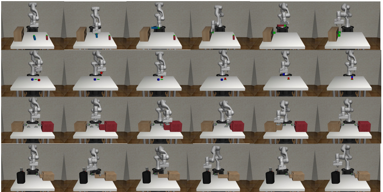
Fig. 7: Task demos. We show the demos of our experiments. We visualize the progress of each task in the Robosuite [12] environment. The first row is PegInHole; the second row is CubeReorder; the third row is HammerPlace; the last row is ServeCoffee.
