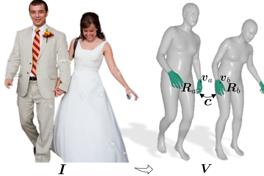
Figure 3: Notation. Given an image I , we can lift each individual into corresponding 3D meshes V . We define contact constraints c as pairs of regions (R_a, R_b) in contact. The loss is defined in terms of the distance between the vertices (v_a, v_b) on the mesh.
