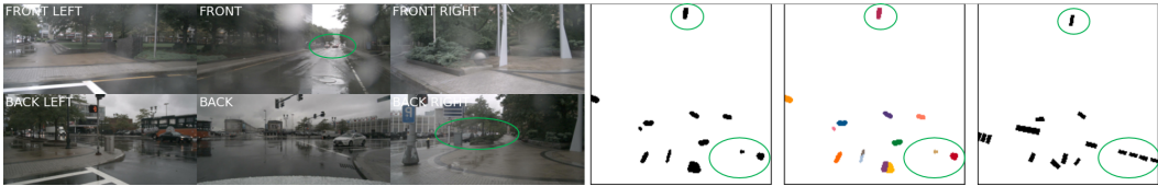
Figure 3: Failure examples on nuScenes [10]. Left shows the six camera views. Right shows our semantic segmentation results, instance segmentation results and the ground truth in turn.
