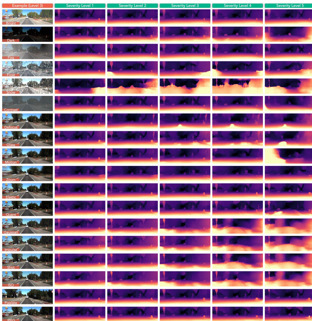
Figure J: Qualitative results of MonoDepth2 [17] under each corruption type across five severity levels. We show examples from the third level in the first column. The lighter regions correspond to near distances and vice versa. Best viewed in color. Zoomed-in for more details.
