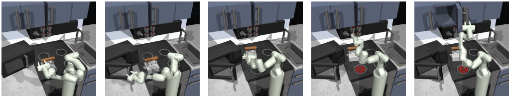
Figure 3: Kitchen environment. The agent is required to perform four subtasks consecutively. Each picture shows the initial position, the robot opening a microwave, moving a kettle, turning on a bottom burner, and opening a hinge cabinet, respectively.
