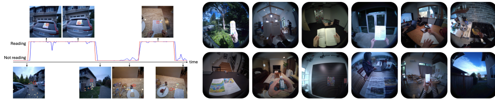
Figure 1: Am I reading? The left figure shows a timeline as the user navigates the world. We aim to solve the task of reading recognition to enable AI assistants in always-on wearables. We identify three modalities: eye gaze (in colored dot patterns), RGB crop around gaze (in red box), and inertial sensors performs the task to high accuracy (with Prediction and GT shown). Images from our Reading in the Wild dataset, which features 100 hours of diverse reading and non-reading activities in real-world settings, with examples shown in the right.
