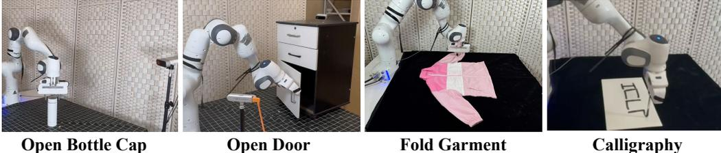
Figure 5: Visualizations of the real-world environments used in our experiments. The tasks are performed using multiple Microsoft Azure Kinect cameras and Intel® RealSense for point cloud fusion and a Panda robotic arm for execution.
