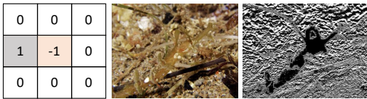
Figure 2: Examples of our BCNN layer. The left is a sample of 3 \times 3 BCNN layer, the center is the input image, and the right is the output of the BCNN layer. Our results show that BCNN can provide a precise boundary for a given image.
