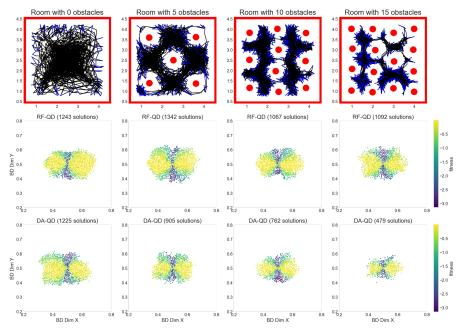
Figure 6: Complex environments with 0, 5, 10 and 15 obstacles. Top: Sample trajectories of hexapod moving with RF-QD. Middle: Example archives by RF-QD. Bottom: Example archives by DA-QD.
