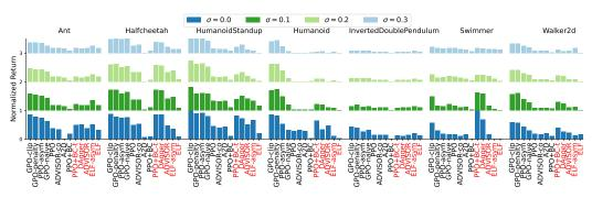
Figure 3: Comparison of GPO and baselines on the Brax domain, where  $\sigma$  represents the scale of Gaussian noise added to the observations. The performance on each task is normalized to [0,1] using the performance of the corresponding pre-trained teacher as a reference. Algorithms highlighted in red are supervised by their corresponding pre-trained teacher.
