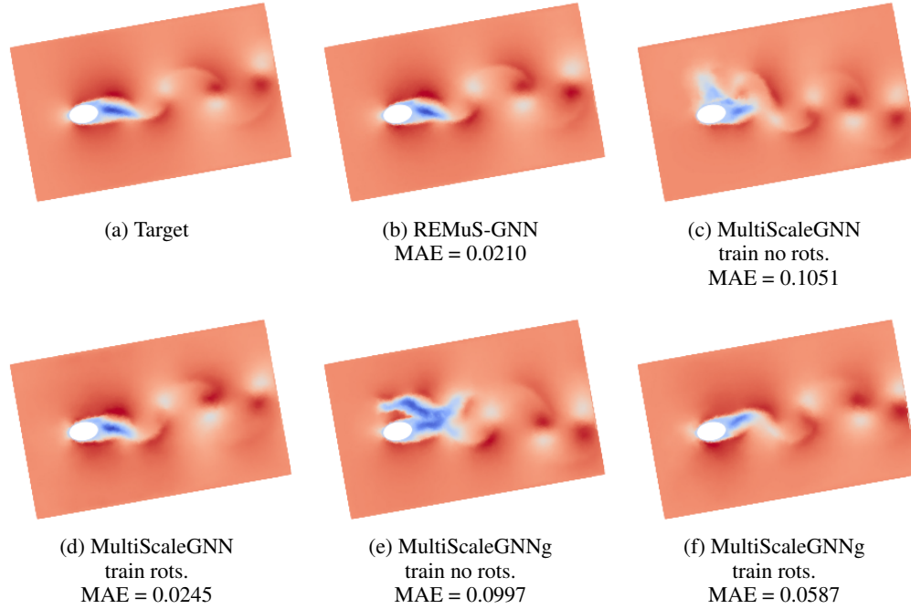
Figure 6: Target and predictions (after 100 time-steps) of the horizontal velocity field with a rotation of 10 degrees of the physical domain (sample from the validation dataset N_{SVal} with Re = 864 ).
