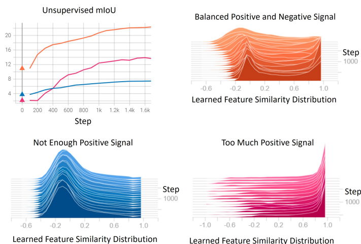
Figure 14: Distributions of feature correspondences between an image and itself across three different hyper-parameter settings. The orange curve and distribution shows a proper balance between attractive and repulsive forces allowing some pairs features to cluster together (the peak at 1) and other pairs of features to orthogonalize (the peak at 0)
