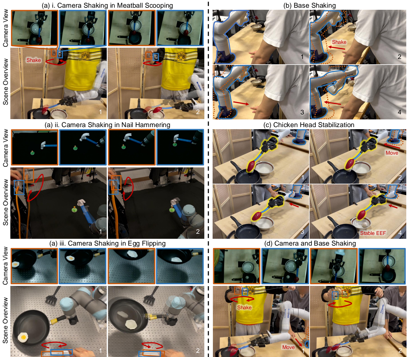
Fig. 5: Robustness to Camera and Base Movement. (a) Camera Pose Robustness: The policy demonstrated the ability to handle camera shaking across three tasks—meatball scooping, nail hammering, and pan flipping. The first row shows the camera view, while the second row provides a scene overview with the shaking motion. (b) Robot Base Robustness: The policy successfully compensated for base shaking, even when the shaking frequency exceeded the robot’s control frequency. (c) Chicken Head Stabilization: At lower base movement frequencies, the end effector displayed a stabilization effect similar to a chicken’s steady head. (d) Combined Robustness: The policy maintained task performance under simultaneous camera and base shaking.
