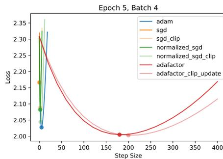
Figure 3: The loss landscape in different update directions on machine translation. The step size is the learning rate normalized by the update step  $\ell_2$  norm.
