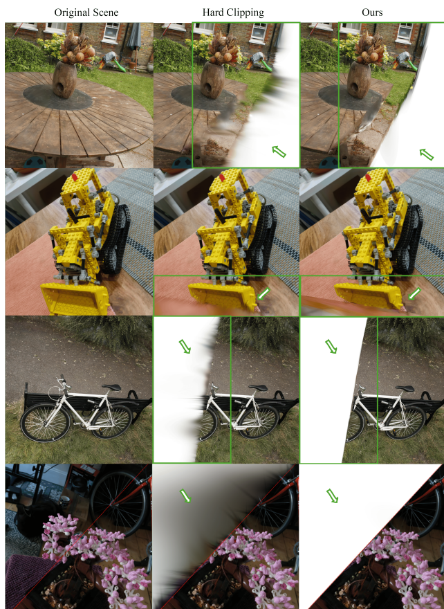
Figure 12. Clipping results on general appearance modeling datasets, showcasing the impact of different strategies near the clipping boundary. Hard clipping introduces spiky artifacts, particularly visible in edge structures. In contrast, our method produces clear contour cutting. The last row shows results on the 360bonsai dataset, where the red line indicates the visualized clipping plane.
