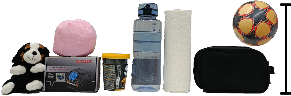
Figure 7: The eight objects we use for grasping experiments shown in Table 1. From left to right: plush toy, styrofoam object, cardboard box, ramen cup, bottle, kitchen roll, pouch, ball. The objects differ distinctly in size, weight, shape and surface friction. The bar denotes a length of 30 cm.
