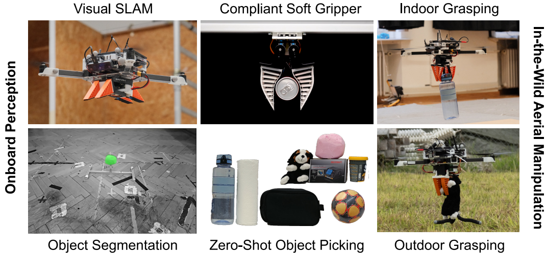
Figure 1: Our autonomous aerial platform demonstrates its aerial manipulation capabilities with onboard-only perception.
