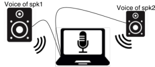
Figure 4: Recording setup for RealTalkLibri data. Two computer speakers imitate two human speakers speaking at the same time to a recording device on the computer.
