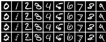
Figure 1: Randomly selected set of non-targeted MNIST adversarial examples generated by EAD. First row: Original, Subsequent rows: \kappa = \{10, 20, 30\} .
