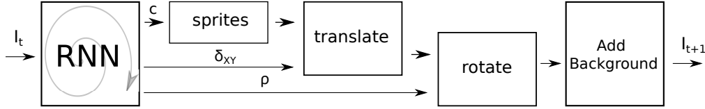
Figure 2: A schematic block diagram for a Perception Updating Network. This configuration uses both convolutions with delta functions for translation and spatial transformers for rotation. It also shows the optional background underlay.
