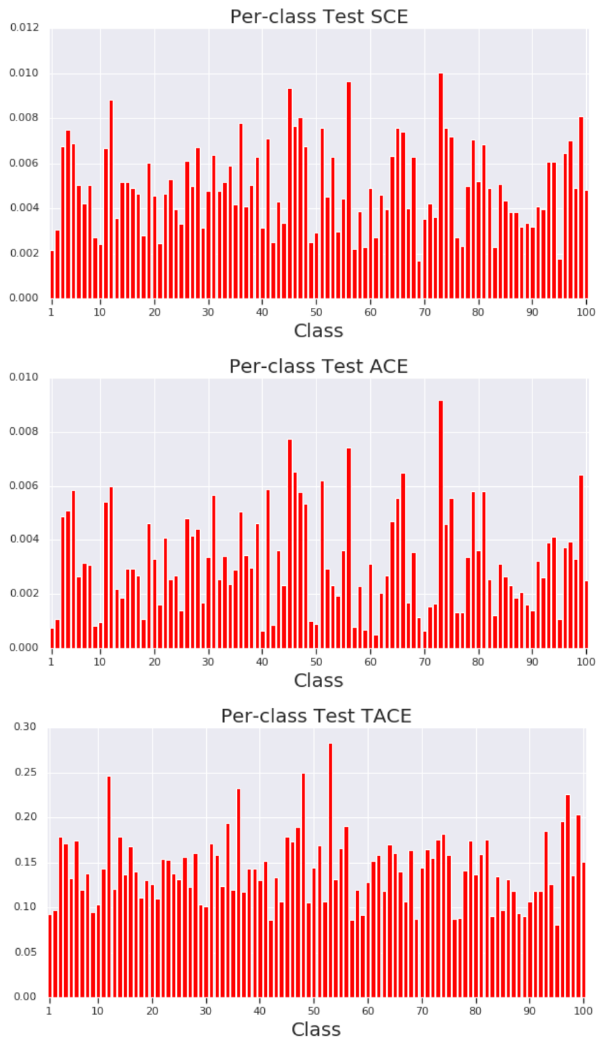
Figure 11: Per-class calibration error for a trained 110-layer ResNet on the CIFAR-100 test set. We observe that calibration error is non-uniform across classes, which is difficult to express with a scalar metric and when measuring error only on the maximum probabilities. Top: Per-class Static Calibration Error. Middle: Per-class Adaptive Calibration Error. Bottom: Per-class Thresholded Adaptive Calibration Error.
