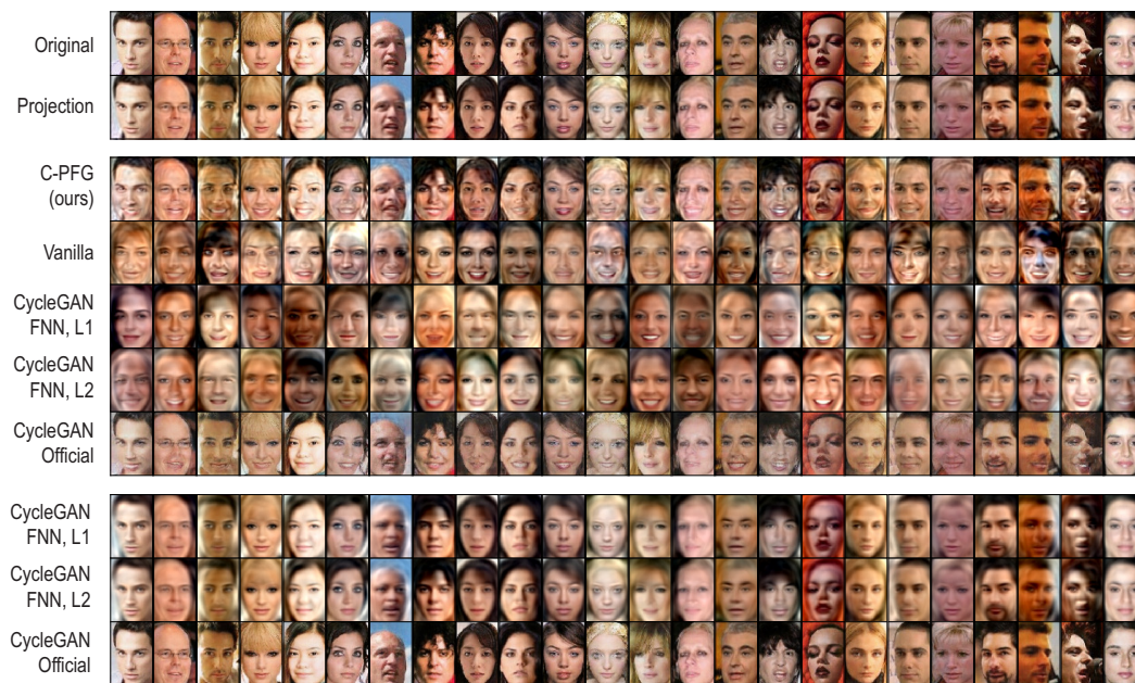
Figure 5: Comparison between our method, vanilla WGAN-GP, CycleGAN with WGAN-GP as GAN loss and L_1 or L_2 loss as cycle-consistency loss, as well as official CycleGAN. The first two rows are the original images and their projections on the 700-dimensional Euclidean space induced by PCA, which are similar. The next five rows are the corresponding outputs. The last three rows are the reconstructed images from different CycleGANs.
