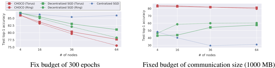
Figure 1: Scaling of CHOCO-SGD with sign compression to large number of devices on Cifar10 dataset. Left : best testing accuracy of the algorithms reached after 300 epochs. Right : best testing accuracy reached after communicating 1000 MB.
