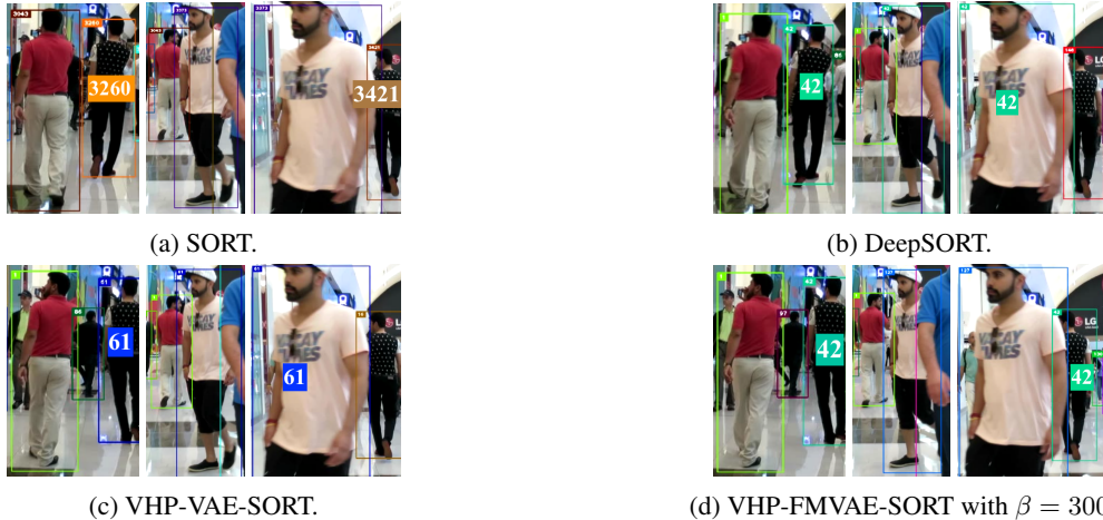
Figure 9: Example identity switches between overlapping tracks. For vanilla SORT, track 3260 gets occluded and when subsequently visible, it gets assigned a new ID 3421. For deeSORT and VHP-VAE-SORT, the occluding track gets assigned the same ID as the track it occludes (42/61), and subsequently keeps this (erroneous) track. For VHP-FMVAE-SORT, the track 42 gets occluded, but is re-identified correctly when again visible.
