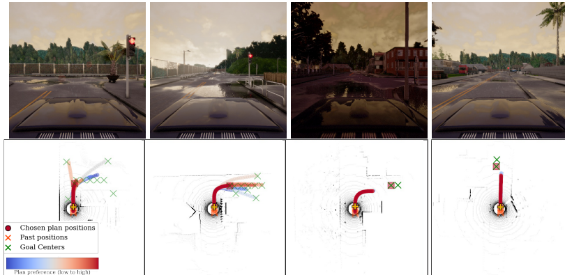
Figure 14: Tolerating bad waypoints. The planner prefers waypoints in the distribution of expert behavior (on the road at a reasonable distance). Columns 1,2 : Planning with 1/2 decoy waypoints. Columns 3,4 : Planning with all waypoints on the wrong side of the road.
