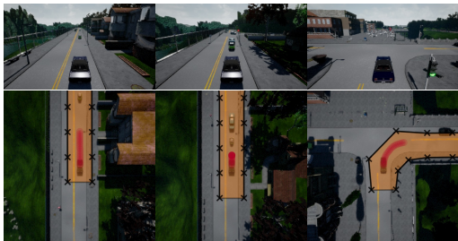
Figure 7: Even with a wider goal region than Fig. 6, the vehicle remains in its lane. Despite their coarseness, these wide goal regions still provide useful guidance to the vehicle.
