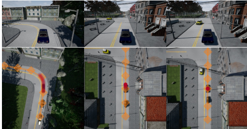
Figure 9: Planning with the Line Segment Final State Indicator yields plans that end along a segment. Orange diamonds indicate line segment endpoints. Red circles indicate the chosen plan.
