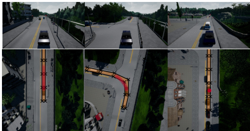
Figure 6: Planning with the Region Final State Indicator yields plans that end inside the region. The orange polygon indicates the region. The red circles indicate the chosen plan.
