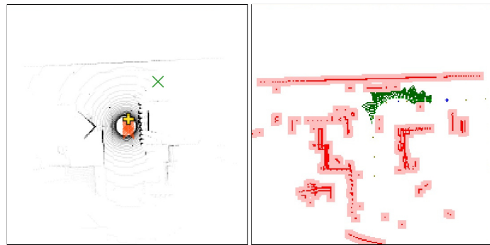
Figure 15: Baseline methods we compare against. The red crosses indicate the past 10 positions of the agent. Left: Imitation Learning baseline: the green cross indicates the provided goal, and the yellow plus indicates the predicted setpoint for the controller. Right: Model-based RL baseline: the green regions indicate the model's predicted reachability, the red regions are post-processed LIDAR used to create its obstacle map.
