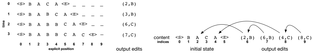
(a) Explicit edit sequence. Left: explicit state at each time. Right: position and content of the edits. (b) Implicit edit sequence. The position components use different indexing from the explicit representation.
