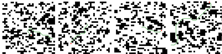
Figure 4: Four example maps and paths from our rock-world dataset. The star shows the goal position with one example path to that goal.
