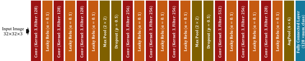
Figure 4: Illustration of the 13-layer Convolutional Network.
