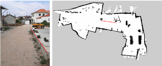
Fig. 6. The important obstacle absent from the map generated by each framework. OCTOMAP (Figure 5 center map) it almost erases the line completely, and RTABMAP (Figure 5 right map) shows only the planters.
