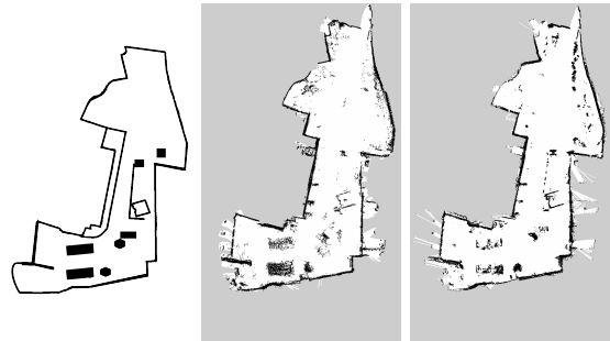
Fig. 5. The map of the ground truth used for the benchmark tool on the left, and the maps obtained by the real world experiments, OctoMap in the center and RTAB-Map right.
