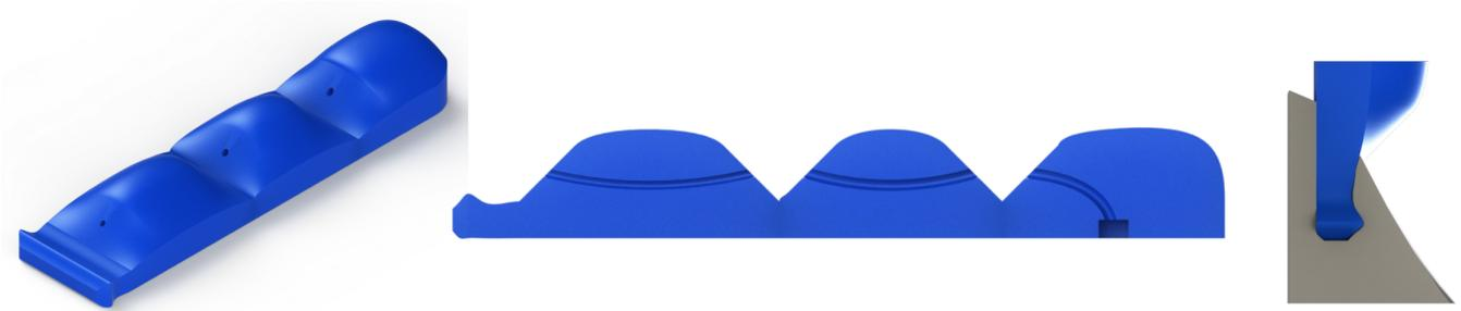
Figure 8: Closeup renderings of an individual finger. Isometric view (*left*), section view (*center*), and detail view of finger detachment (*right*).
