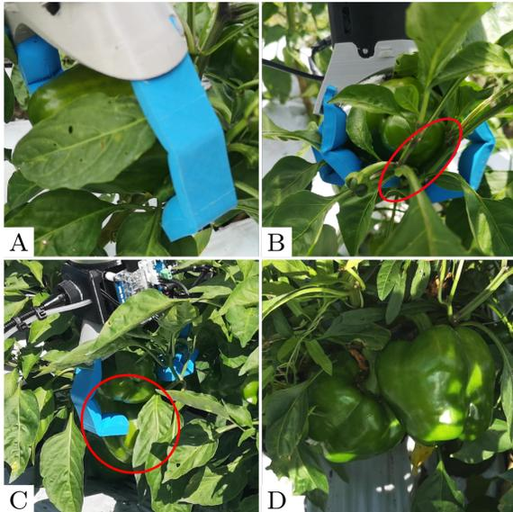
Figure 6: Case study of 4 failure cases: A: Foliage. B: Plant stem in contact with fruit, grasping fails. C: Peppers are too close together. One finger gets lodged on the adjacent fruit causing the grasp to fail. D: Example of two peppers growing very close together behind thick foliage.
