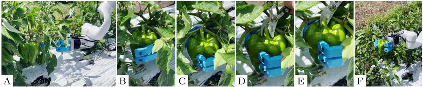
Figure 3: Successful harvesting sequence of teleoperated robot system. A: The robot approaches a pepper plant. B: Gripper moves into a pre-grasp position. C: Gripper closed, successfully grasping the pepper. D: Manually position the cutting mechanism at the fruit stem. E: Stem cutting. F: Retract arm to retrieve pepper.
