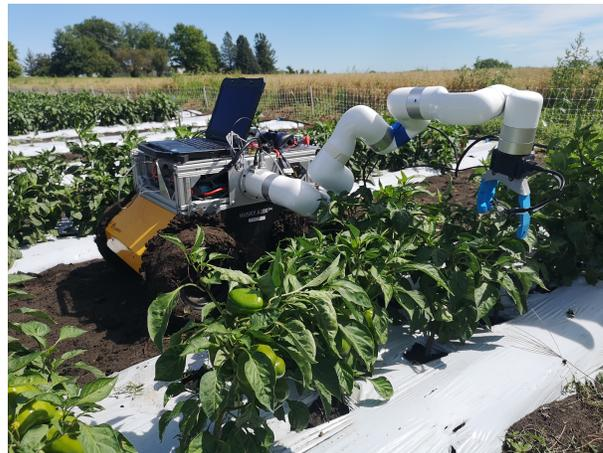
Figure 1: Green Pepper harvester robot prototype in the field: Mobile base, robot arm, and fully printed soft gripper with cutting mechanism.
