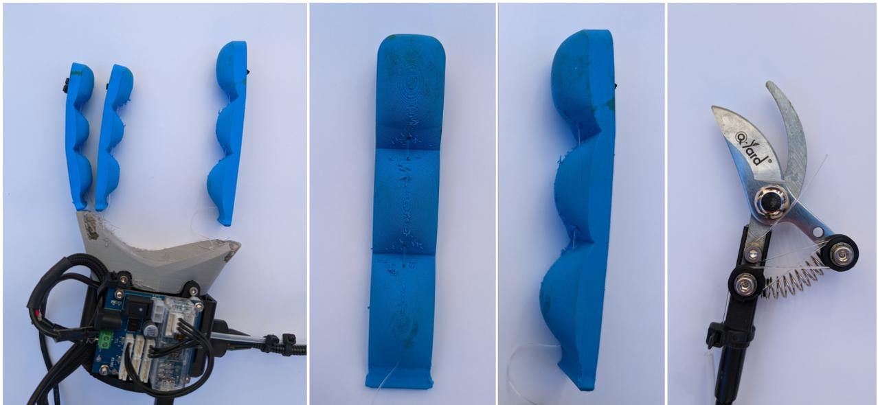
Figure 9: *Left*: Gripper with detached fingers. *Center*: Closeup of individual finger, printed from TPU material. *Right*: Closeup of cutting device.
