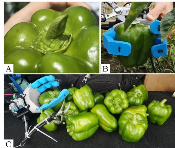
Figure 4: A: Clean cut achieved by pruning blades of gripper. B: Stable grasp of a pepper. C: Gripper and a subset of harvested peppers; no pepper was bruised by the gripper.
