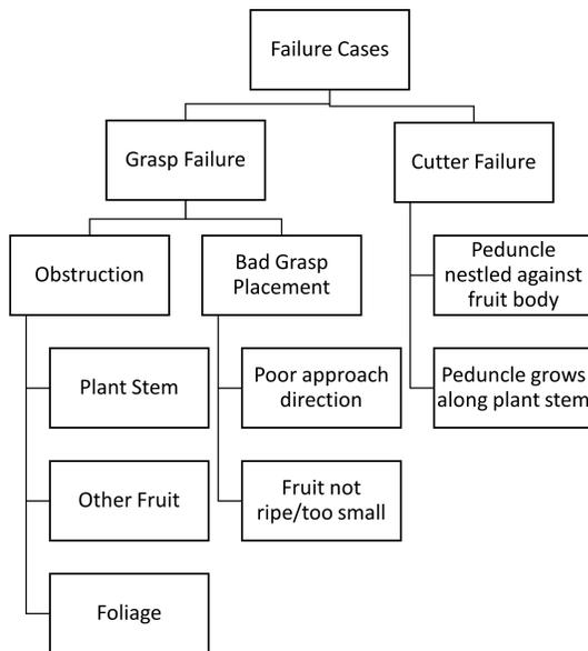
Figure 5: Classification of end-effector failure cases that are observed during our robotic harvesting case study.
