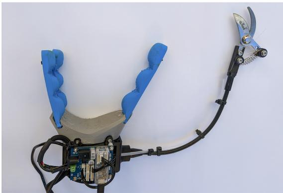
Figure 2: Fully printed soft gripper and cutting mechanism. The three detachable fingers and cutting shears are driven by servo motors enclosed in the wrist via tendons.
