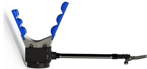
Figure 7: CAD rendering of end-effector design.
