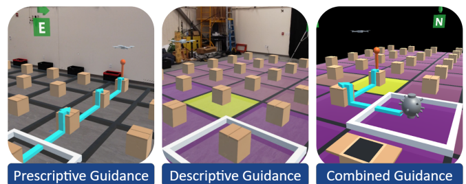
Fig. 1. AR-based visual guidance modalities: prescriptive guidance, featuring arrows and pins (left), descriptive guidance, featuring an environmental heatmap (middle), and a combination of both guidance types (right) in an experimental Minesweeper-inspired domain.
