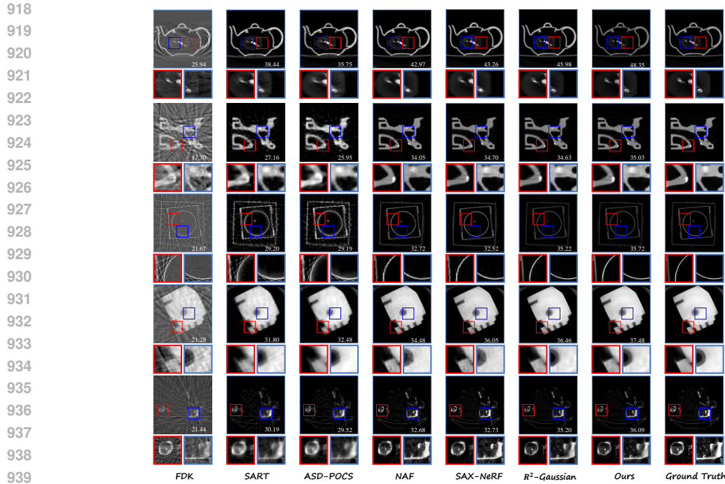
941 Figure 10: The figure shows CT reconstructions from the X-3D dataset , covering artificial objects 942 (teapot, engine, present, mount, and backpack) categories. All under 25-view conditions. 943 944
