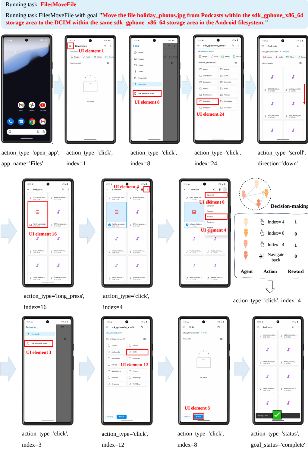
Figure 3: An example of task execution steps of CollabUIAgents mobile which is trained on Qwen2 7B and facilitates 4 agents engaging in 3 rounds of conversation. "action.type" represents the action taken, and "index" represents the index of the UI element. The positions of the relevant elements on the UI interface are marked in red.
