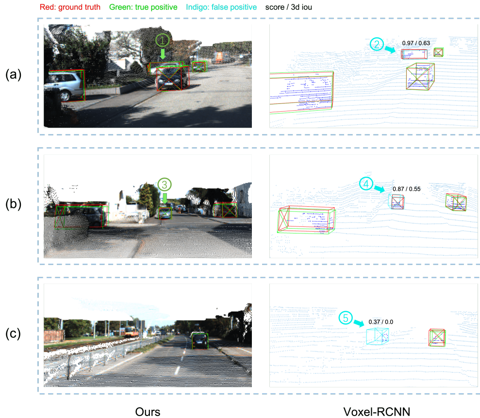
Figure 9: Comparison between SFD and Voxel-RCNN. For the visualization of SFD and Voxel-RCNN, we use pseudo clouds and raw clouds, respectively. We show true positives, false positives and ground-truth boxes in green, indigo and red, respectively. The raw LiDAR points inside prediction boxes are rendered in blue. Green arrows represent that our predictions are more accurate, and indigo arrows represent false positives of Voxel-RCNN.
