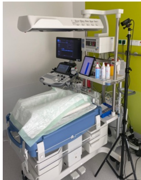
Figure 12: Data Acquisition Setup. The child is placed into a positioning cradle to minimise movement during scanning. Ultrasound probe movement can be tracked using a tracking camera (right) while imaging results are displayed in a screen above the cradle.
