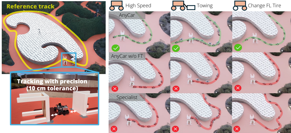
Figure 1: Performance of AnyCar and baselines in the wild under state estimation errors. Above: A 10 cm tolerance corridor is set as a checkpoint. Below: each row represents the true trajectory of one method, and each column corresponds to a specific setting for the 1/16 scale car: high speed (2 m/s), towing a box, and replacing the front left tire with a plastic wheel. All settings significantly alter the vehicle dynamics.
