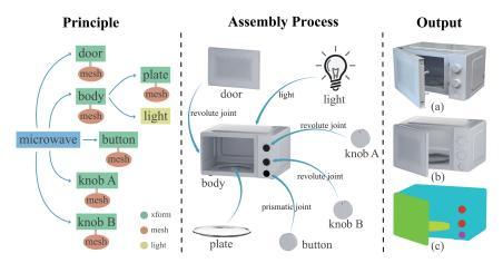
Figure 2: An asset in ArtVIP. Left: Top-down assembly principle. Middle: Assembly process. Right: Comparison between the real object (a) with its digital-twin (b), and annotations (c).
