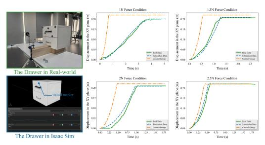
Figure 6: **Left:** Digital-twin asset examples in real-world and simulation. **Right:** Analysis of the drawer's displacement driven by different forces.
