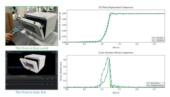
Figure 12: **Left:** Digital-twin asset examples in real-world and simulation. **Right:** Analysis of the oven's displacement.
