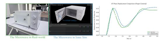
Figure 11: **Left and Middle:** Digital-twin asset examples in real-world and simulation. **Right:** Analysis of the Microwave's displacement.
