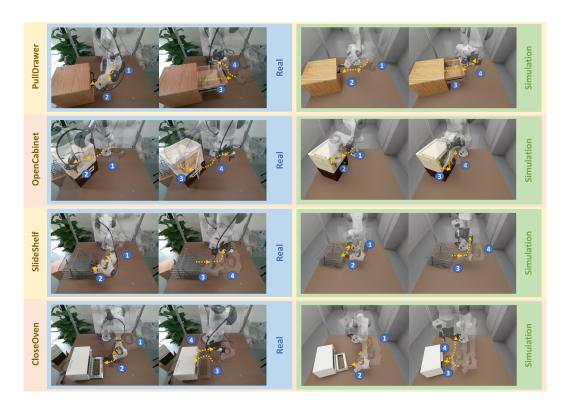
Figure 13: The four articulated-object manipulation tasks conducted for imitation learning.
