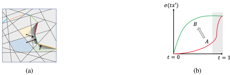
Figure 2: (a) A geometric view of the input space in a ReLU network. Dashed lines correspond to activation constraints while the colorful solid lines are piece-wise linear decision boundaries. Taking gradient of the model’s output with respect to the input returns a vector that is orthogonal to a nearby boundary (points in the blue and green regions) or an extension of a nearby boundary (the point in the yellow region). (b) Curves of the model’s sigmoid output \sigma(tx') (y-axis) against interpolation parameter t (x-axis).
