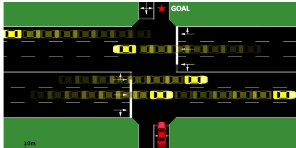
Figure 3. Challenge Scenario. The DQN policy begins accelerating in anticipation of the clear path. TTC would have waited until all cars were clear, missing the opportunity.
