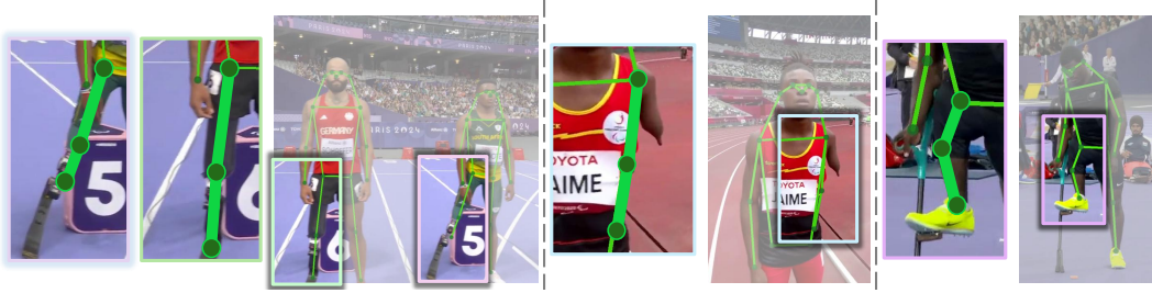
Figure 2: Examples of keypoint predictions by the ViTPose base model trained the COCO dataset. Left: prostheses are erroneously predicted as natural ankles, leading to false right-ankle detections. Middle: the model fails to localize the residual limb end and places the left-wrist keypoint on the torso. Right: pronounced asymmetry in thigh length results in the right-knee keypoint being placed at an anatomically implausible midpoint between hip and ankle. These cases show limited generalization to limb differences.
