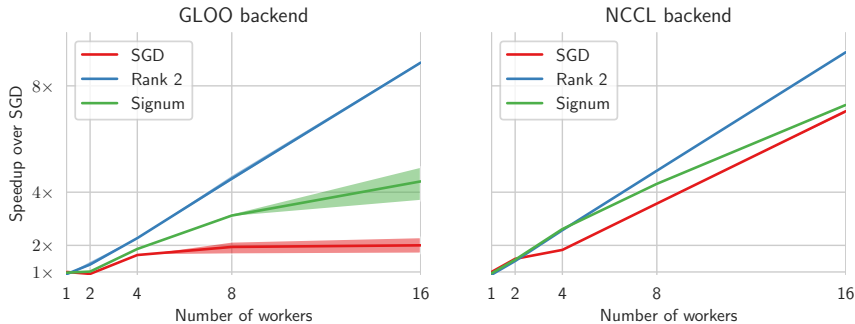
Figure 3: Scaling of POWERSGD on CIFAR10 compared to full-precision SGD and Signum (Bernstein et al., 2019) on two communication backends. The batch size increases linearly with the number of workers. We compare training time for one epoch to 1-worker SGD. Note that the faster NCCL backend used throughout benefits the baselines more than our method.
